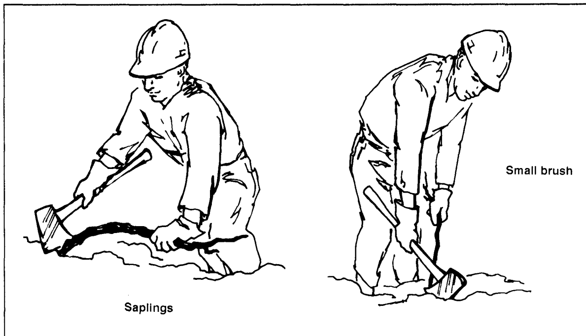
Figure 5-4. Clearing away small brush and saplings
