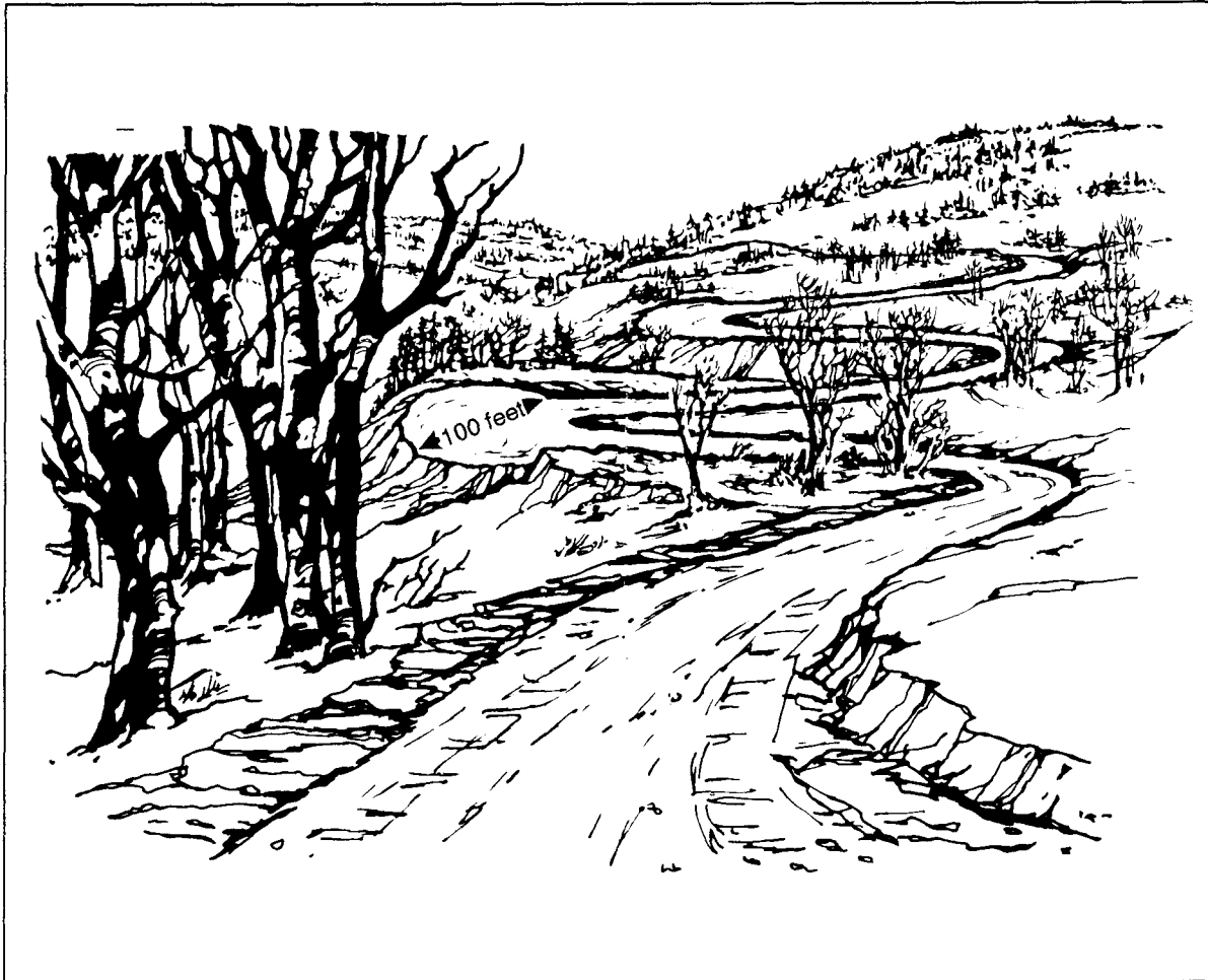
Figure 4-6. Development of switchbacks
